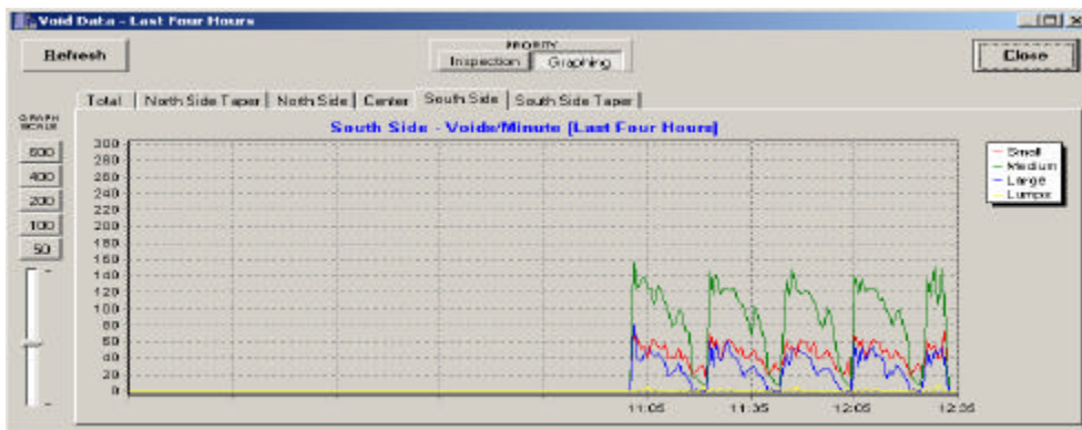
Charting of voids per minute for the whole board and each of the five user-defined zones.
